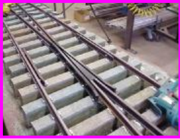
New Steel switch frog
