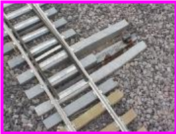
Some main line switches have the 'big throws' on them, the arrow indicates it's direction. These have 'lot's' of leverage, please don't force them!
