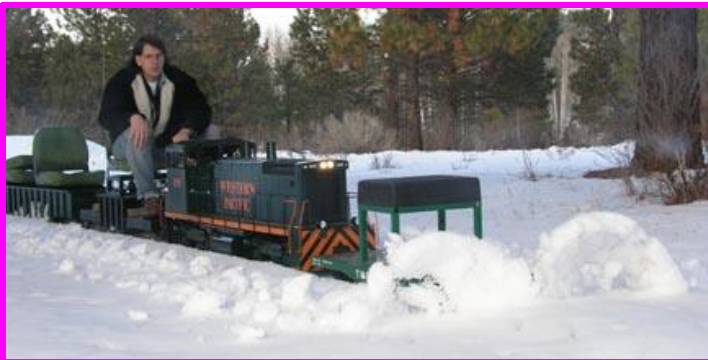
Ron Young's plow is just amazing. He has designed the best so far and it works like a dream. Check the snow flying as Tom Vertel plows the tracks near his home. The plow mounts in the coupler pocket of a riding car. ED
