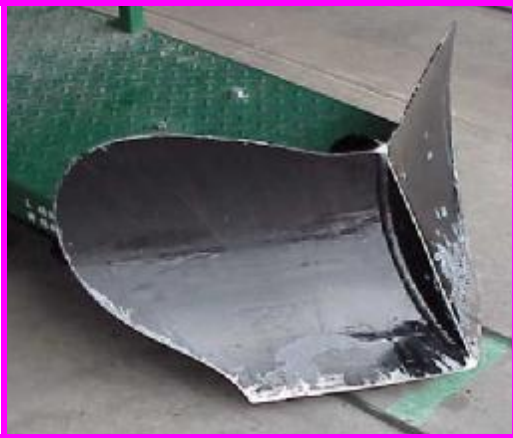
Ron Young's plow is just amazing. He has designed the best so far and it works like a dream. Check the snow flying as Tom Vertel plows the tracks near his home. The plow mounts in the coupler pocket of a riding car. ED
