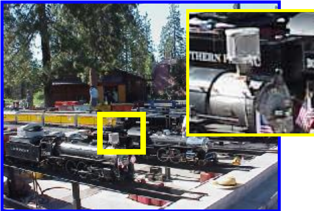
Spark arrestors were used during the Triennial and here is a good example. Unless you want to spend some of your valuable Train Mountain time building one, you might want to build yours at home and bring it with you.
