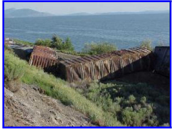
The previous picture was the middle of the errant train while the picture above was caused by a couple of helpers at the rear that helped a little to much.
