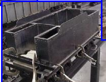
Lee Brooks' much improved loading plates for use on the Crisp Yard lifts. Now that's heavy duty!
