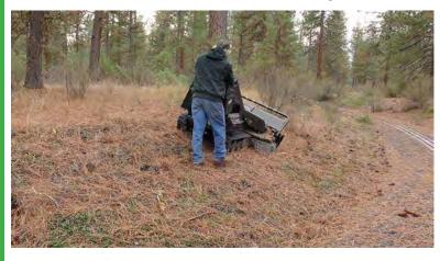
In this image, Richard is demonstrating how well the Brush Blazer does running along a side-hill. There is a limit, as at some point you tend to slide sideways down the hill. The alternative is to then run the Brush Blazer up and down the hill, but this is a lot more work and not nearly as efficient.
