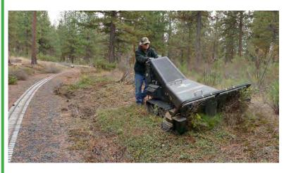
For this demonstration with the Brush concentrating Blazer, we are on increasing the visibility around corners. The further the engineer can see, the sooner the engineer can react. With all other factors being equal, the sooner the engineer can react - the sooner the train can be stopped.
