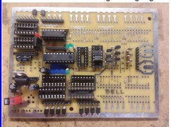
boards fabricated professionally, but Dave and I did all the part placement and soldering. Lightning protection is integrated onto these boards, and all of the components are all socketed which helps immensely in diagnosis and repair of problems.
